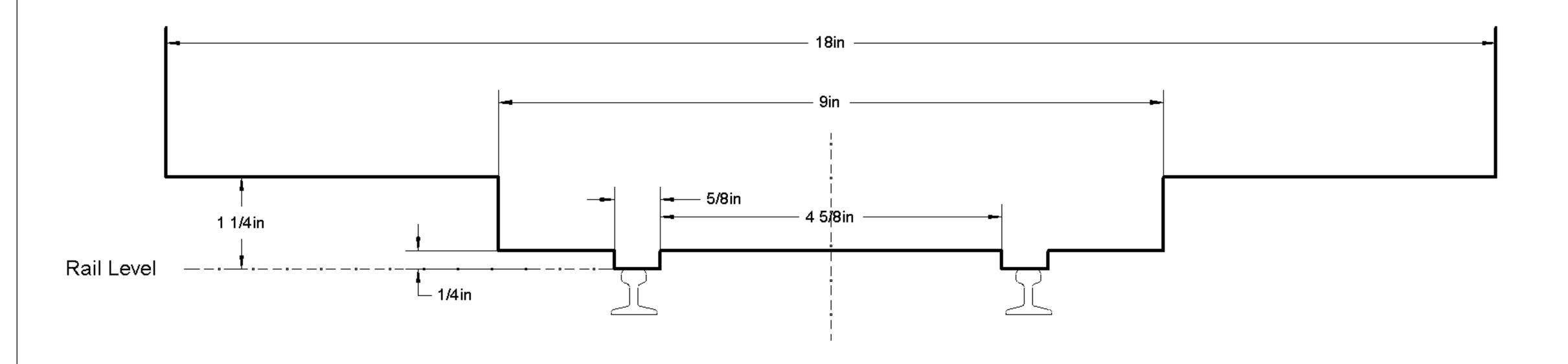
Note, no part of any vehicle may be below this profile at any time, due allowance must therefore be made for any lowering of a vehicle when loaded.
